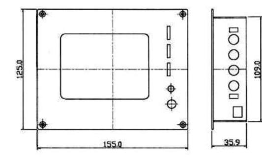
Line Drawing for: Model No. LM412 All sizes are in mm Drawing not to scale.
