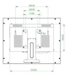
Line Drawing for: Model No. L151AVL All sizes are in mm Drawing not to scale.
